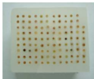
Fig.7 The TMA paraffin block constructed by our ZM-1 tissue microarrayer
